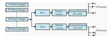
Figure 2: frame work flow chart
