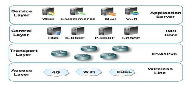
Figure 1: IMS layered architecture.
