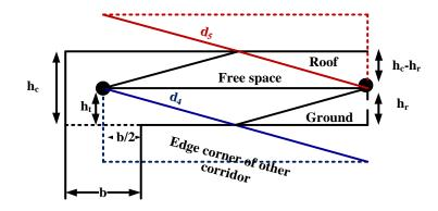
Figure 3: Free space and the reflective rays from the ground and roof
