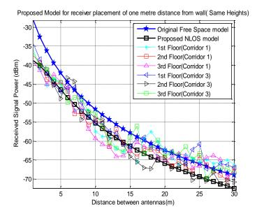
Figure 7: The comparison results of proposed model, original free space model and experimental data for corridor (1) and (3)
