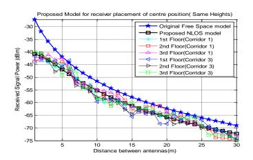
Figure 6: The comparison results of proposed model, original free space model and experimental data for corridor (1) and (3)
