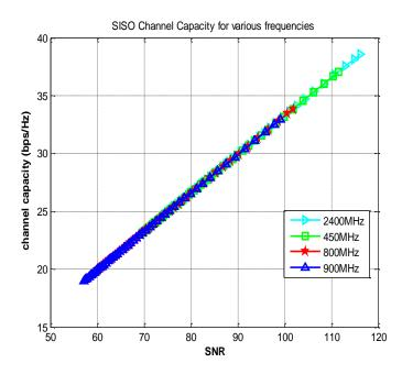
Figure 11: The channel capacity values for four types of frequencies
