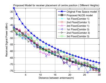
Figure 8: The comparison results of proposed model, original free space model and experimental data for corridor (1) and (3)
