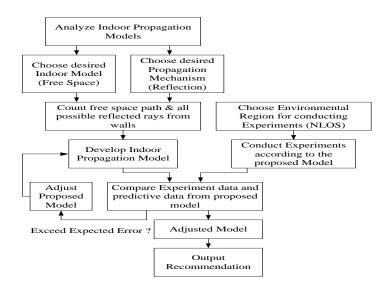
Figure 2: System Block Diagram of Proposed Mode
