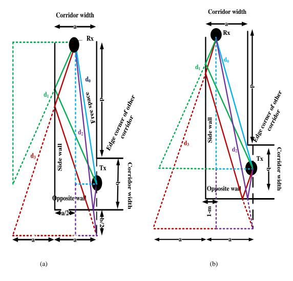
**Figure 4**: (a) The reflective rays from the side and opposite walls while the receiver located at center point (b) The reflective rays from the side walls and opposite walls while the receiver located one meter from side wall.
