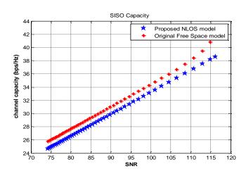
Figure 10: SISO Channel Capacity for free space and proposed model
