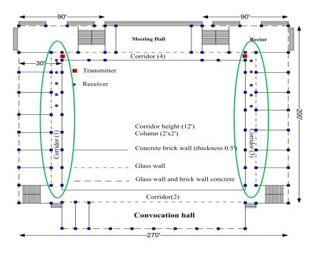
Figure 5: Building Layout of experimental region
