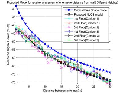
Figure 9: The comparison results of proposed model, original free space model and experimental data for corridor (1) and (3)
