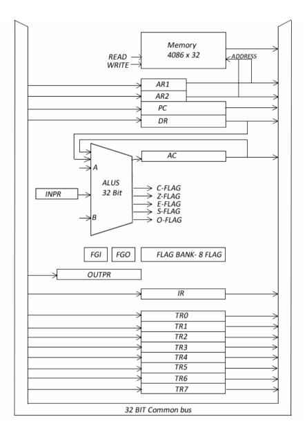
Figure 1: Register and ALSU configuration (RC2)
