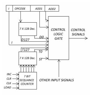
Figure 2: control unit configuration of rc2
