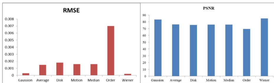
**Figure 5:** RMSE and PSNR values linear and non-linear filter
