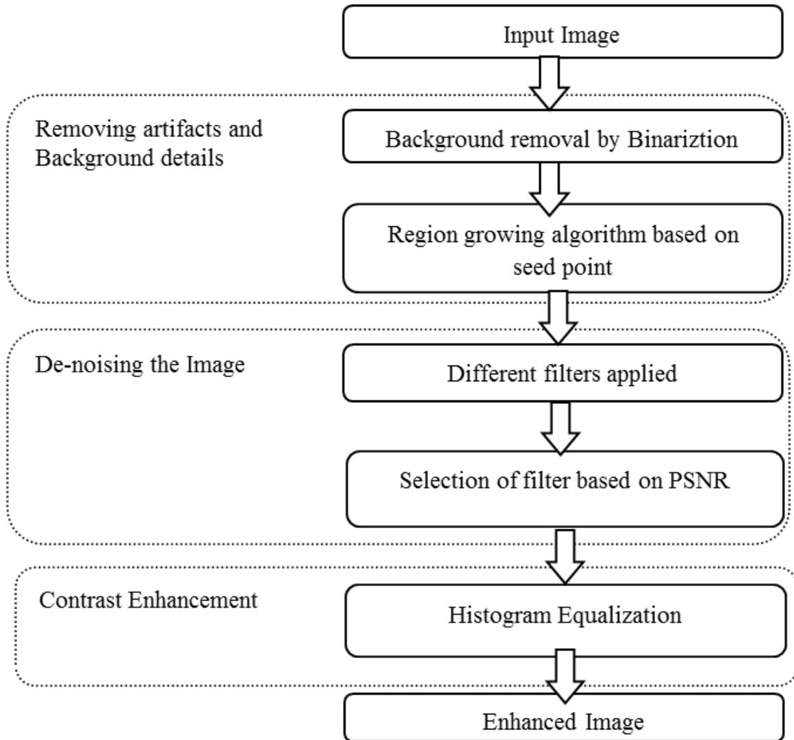
**Figure 1:** Flow of proposed method.
