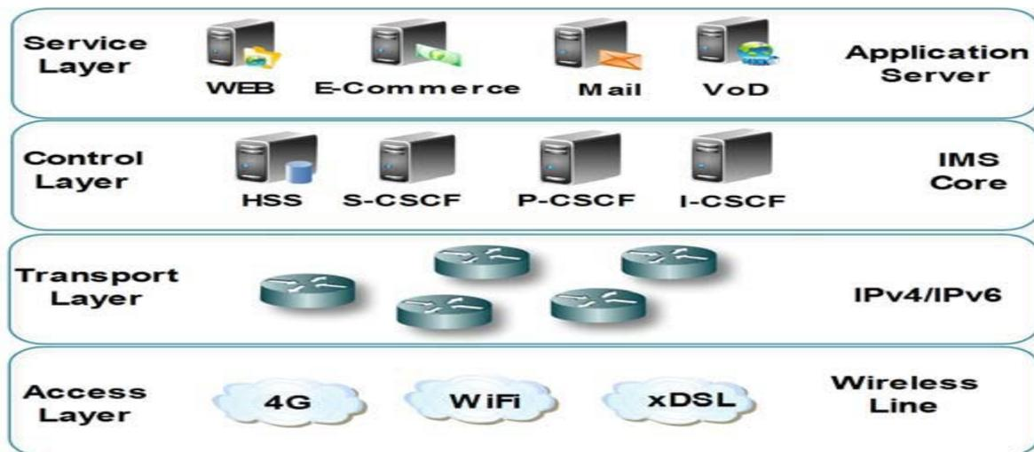
**Figure 1:** IMS layered architecture.
