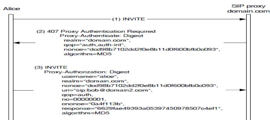
Figure 5: Digest operation
