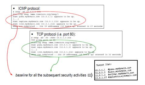
Figure 1: Example of port mapping
