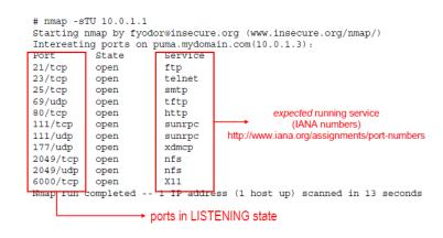
Figure 2: Example of network mapping (using nmap)
