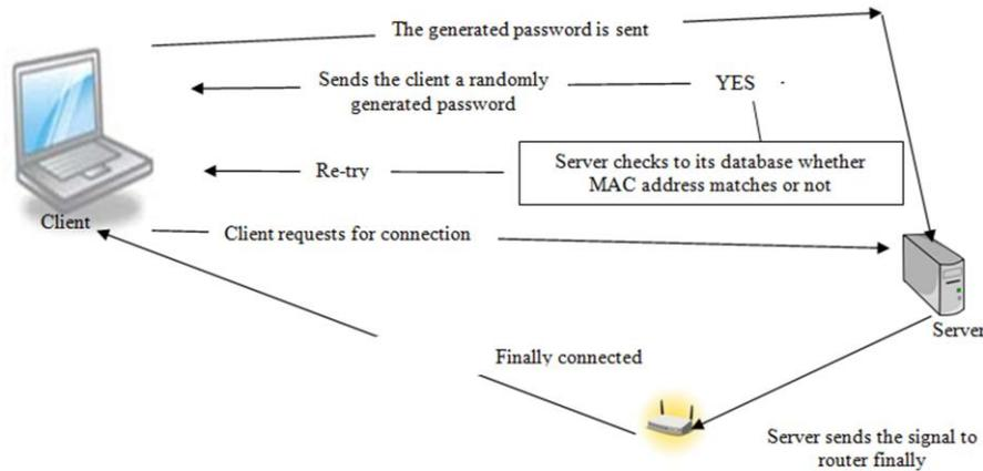
**Figure 5:** Experimental operation of the proposed protocol, with the request from left to right
