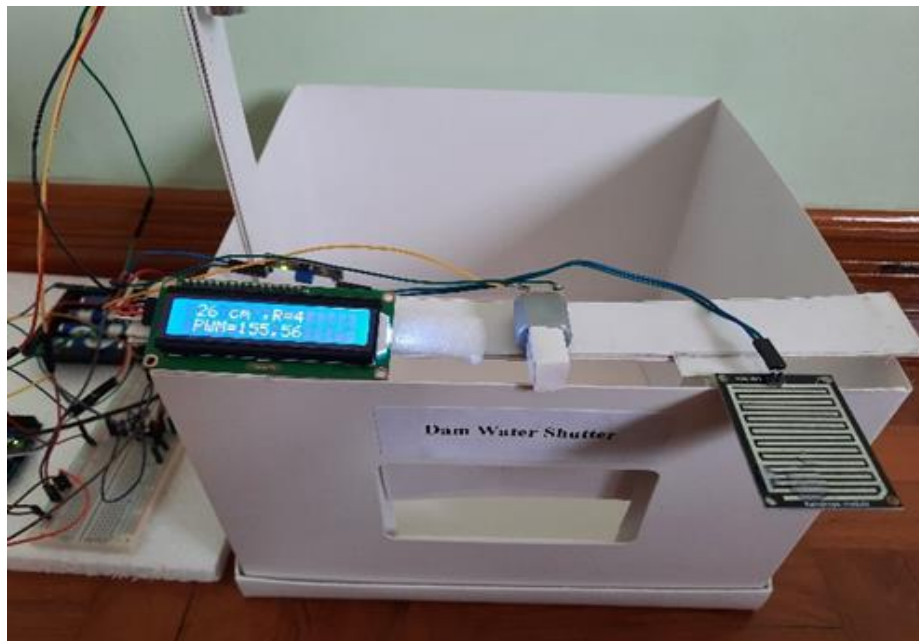
Figure 9: Small Skill Model of Water Dam Shutter
