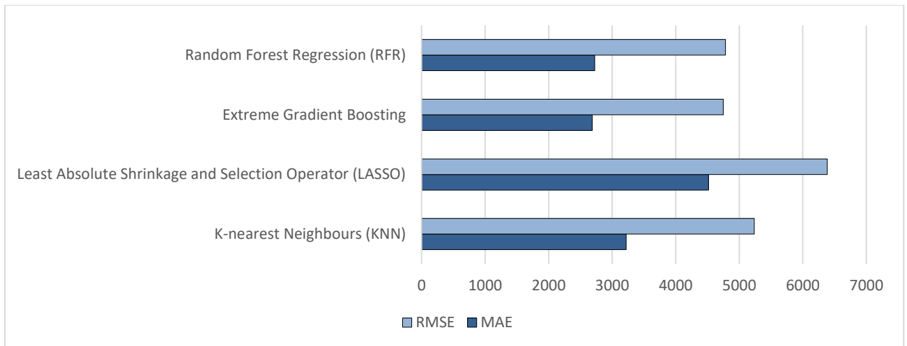
Figure 9: Comparison of the four (4) models, on two performance measures (RMSE and MAE)
