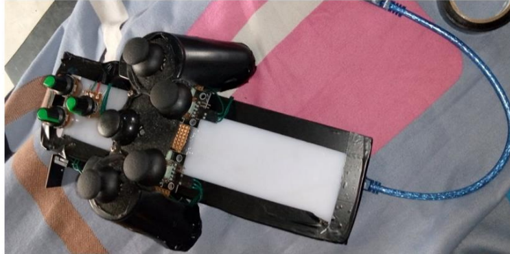
Figure 16: Assembly of the joysticks and potentiometers
