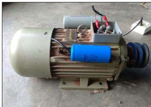
Figure 2: One phase capacitor start induction motor
