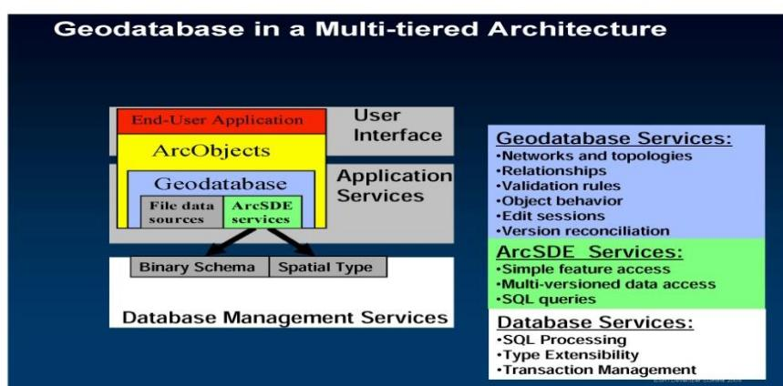
Fig. 3: Geodatabase in a Multi-tiered Architecture
