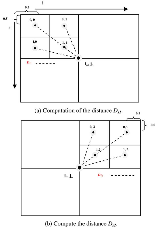
**Figure 2:** Schematic description for for computing the distance DS for cases (a and b), which are similar to cases (c and d).
