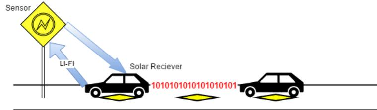
**Figure 1:** Communication between Road Side Unit and fitted LED
