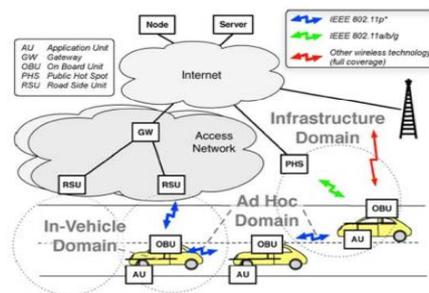
Figure 5: Ad-hoc network for V2V communication
