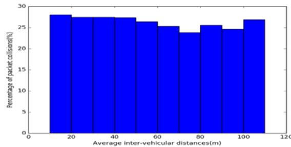
**Figure 5:** Average % of collisions vs. average inter-vehicle distance
