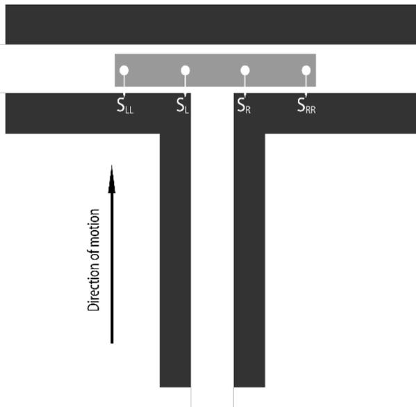
Figure 15: T-junction detection
