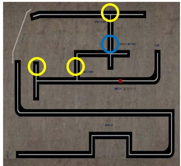
Figure 16: T-junctions and + junction on track
