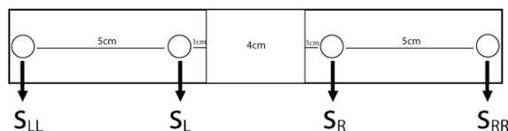
Figure 5: Sensor array
