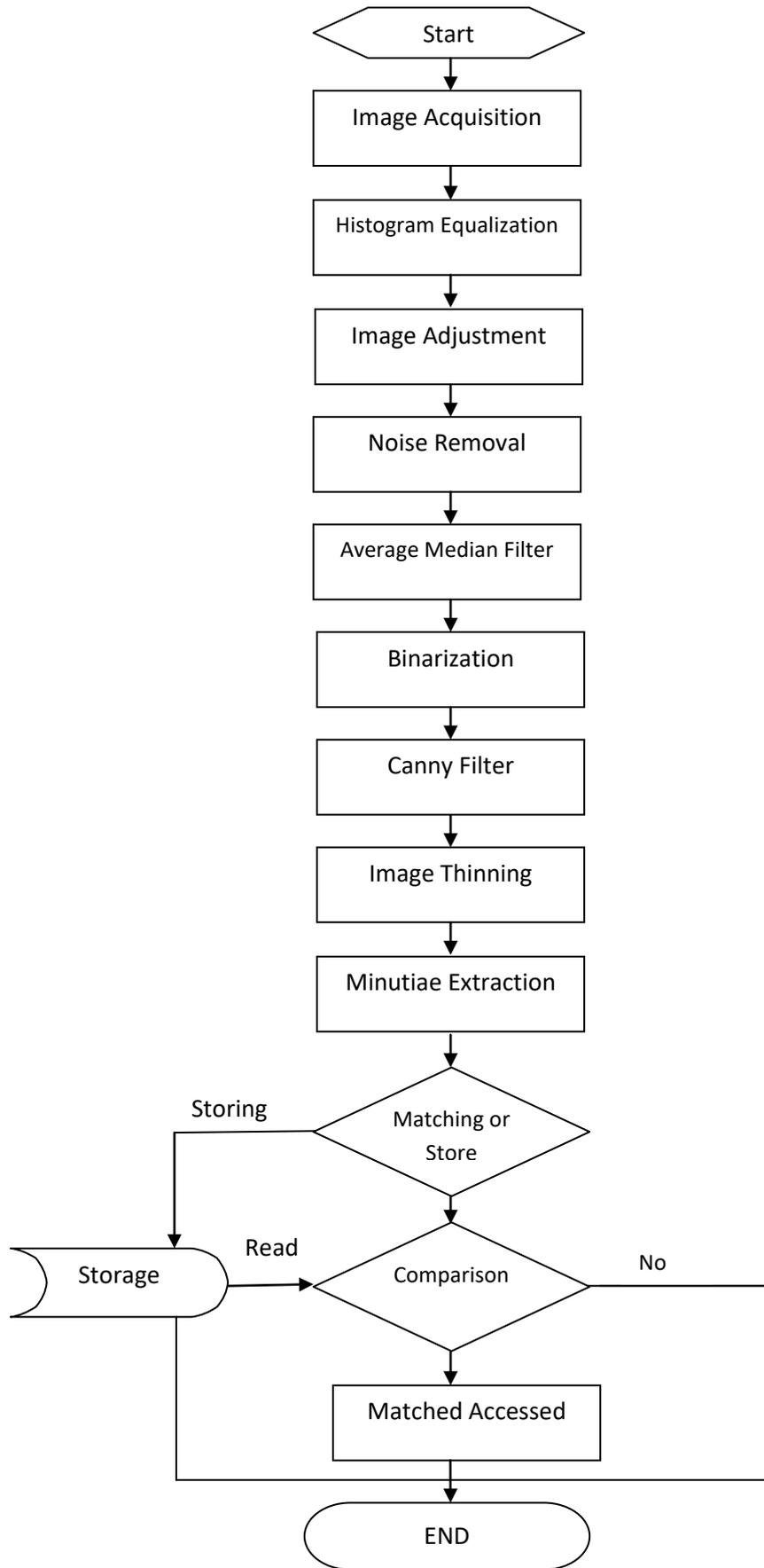
Figure 2: proposed framework for enhancement of the fingerprint image.
