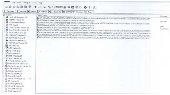
(c) Attack Successful on SHA 256 but not successful on SHA 512. The password column on Cain and Abel reveals the plain text of data hashed with SHA 1 but for data hashed with SHA 512, the password column is blank ( Attack on SHA 512 unsuccessful)
